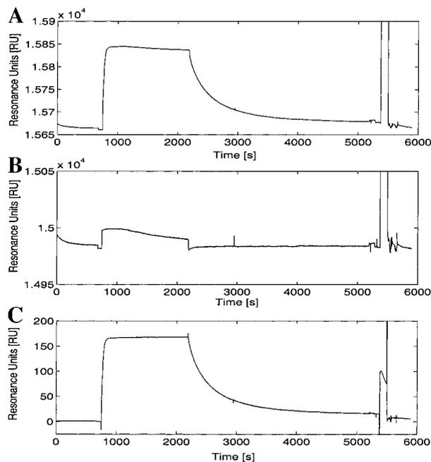
**FIG. 3.** Sensorgram of one of the 100 nM injections for the D1.3 Fab–HEL experiments (see text) including stripping signal. (A) Measured sensorgram. (B) Reference cell sensorgram. (C) Sensorgram after reference cell subtraction.
