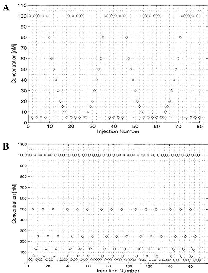
**FIG. 1.** A graphical representation of the injection levels for the experiments discussed under HEL–D1.3 Fab interaction (A) and I-A<sup>u</sup>:10.2.16 Fab interaction (B). The  $x$  axis of the plots shows the number of the injection, whereas the  $y$  axis shows the concentration of analyte that is being injected. The concentration levels of HEL used were (A) 5, 10, 15, 20, 30, 40, 50, 60, 80, and 100 nM and of 10.2.16 Fab were (B) 33, 67, 133, 250, 500, and 1000 nM.
