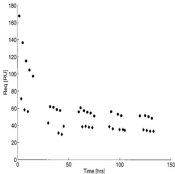
**FIG. 2.** Measured equilibrium values as a function of time for the experiment (see text for more details) in which a CM5 chip was coupled with D1.3 Fab and HEL was flowed across the chip with flow rate  $10 \mu\text{l}/\text{min}$ . The depicted measurements were obtained in flow cell 3 for injection concentrations of 5 nM ( $\blacklozenge$ ) and 100 nM ( $\bullet$ ). The decrease in measured equilibrium values for these repeat injections is clearly visible.
